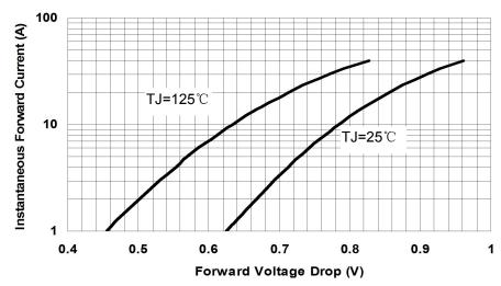
Fig.3-Typical Instantaneous Forward Voltage Characteristics
